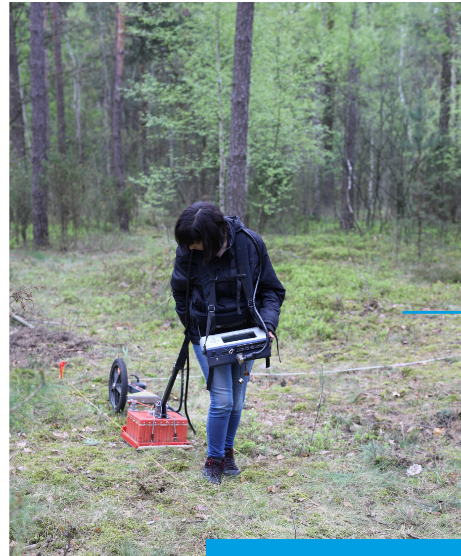
GPR (Ground Penetrating Radar) survey in the forests around the execution site at Treblinka labour camp at the site of possible unmarked mass graves. Copyright @ Centre of Archaeology, Staffordshire University.
